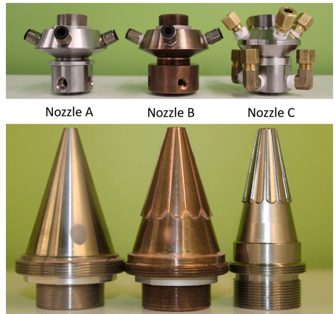
Fig. 5. Prototyped versions of each nozzle that were both simulated and tested experimentally.
