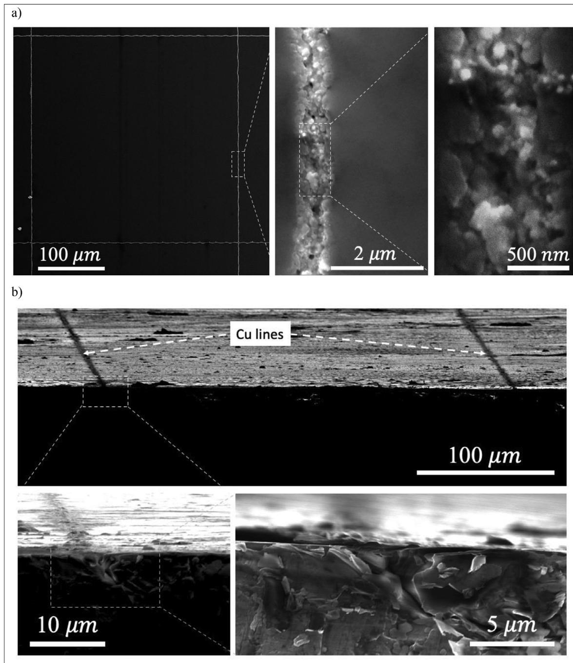
Fig. 2. SEM images of the copper grid: a) surface view, b) cross-sectional view.
