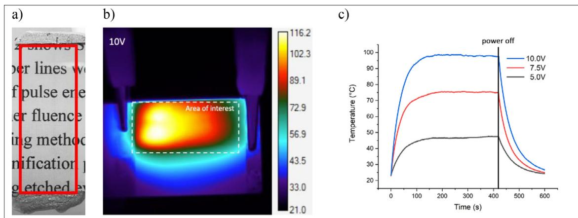
**Fig. 3.** a) Optically transparent heater, b) A thermal camera image. (The average temperature inside the area of interest is 97.6°C), c) The temperature profile of the heater for different voltages.
