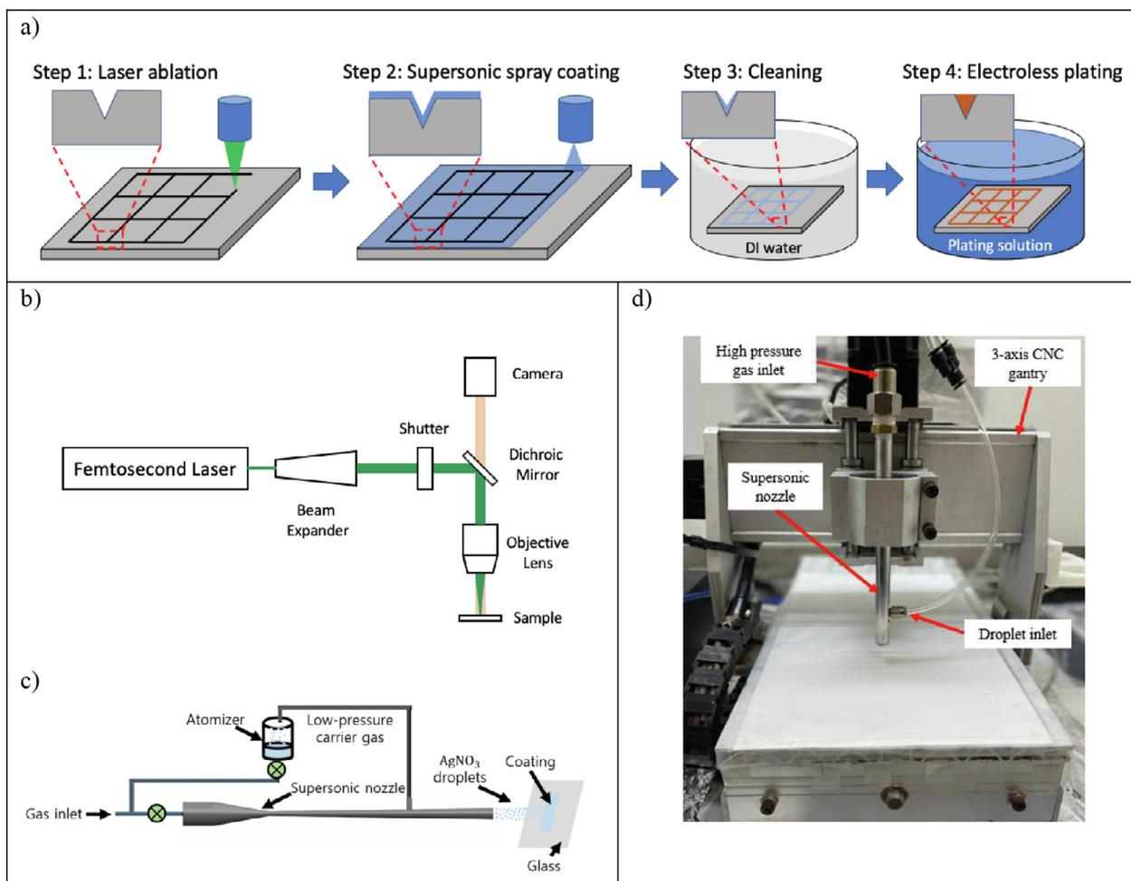
Fig. 1. Schematic of (a) the fabrication procedure, (b) the laser setup, (c) the supersonic spray deposition system; (d) experimental setup of the spray deposition system.
